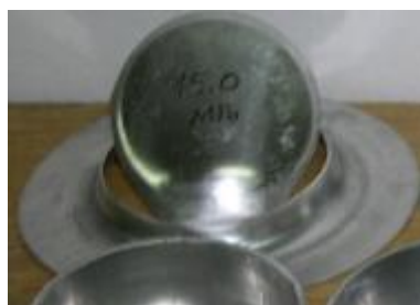
Figure 2: Ruptured vessel image
