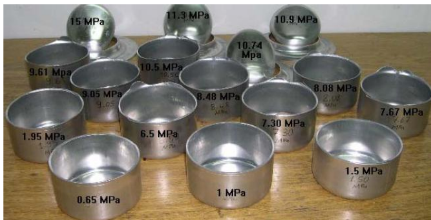
Figure 5: The properly formed vessels and ruptured vessels because of the heigh BHP
