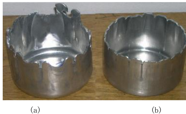
Figure 1: Wrinkled vessel samples. a) without blank-holder b) low blank holding
