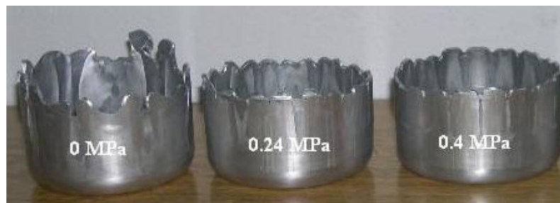
Figure 4: Wrinkled vessels because of the low BHF
